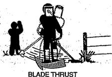
PROPER BLADE - USE ONLY THE 8 3/4 INCH SAW BLADE OR 10 INCH BRUSH TRI-BLADE AND PROPER HARDWARE AS SHOWN. THE USE OF ANY OTHER PARTS CAN RESULT IN SERIOUS INJURY. DO NOT USE ANY ACCESSORY OR ATTACHMENT OTHER THAN THOSE RECOMMENDED BY THE MANUFACTURER FOR USE WITH THIS UNIT. BLADES THAT ARE BENT, WARPED, CRACKED, BROKEN, OR DAMAGED
